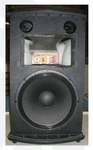
This is what it looks like with the grill and horn assembly removed. See the next page for further instructions and additional pictures on how to remove and replace the high frequency driver.
